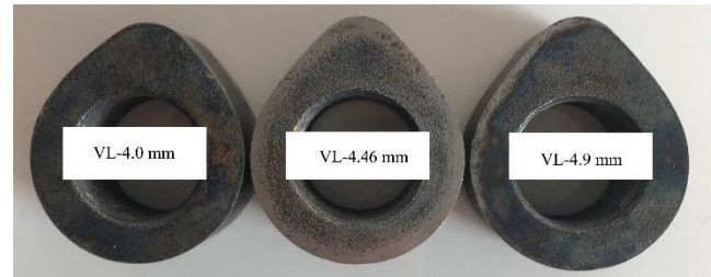
Fig. 8. Cam profiles with different valve lift amounts produced on CNC wire erosion machine.
