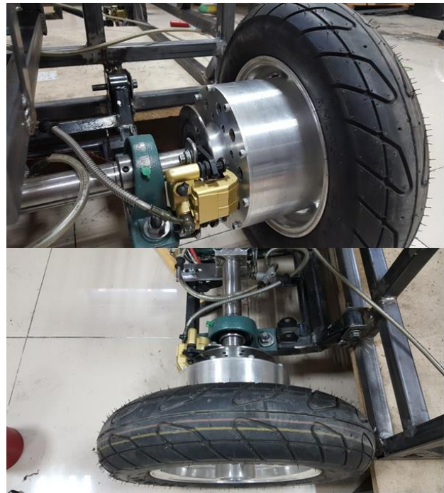
Figure 19. Mounting of the motor to the vehicle
