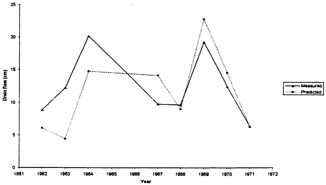
Figure 2.12. Predicted (using van Schilfgaard eq. based K_{sat} ) and measured total cumulative drain flows (183 days) at the drainage experiment of OARDC North Central Branch, near Sandusky, Ohio (Schwab et al., 1963; 1975; and 1985).
